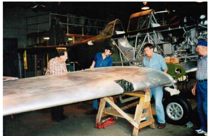
Wings Go On 2001 – Placing right wing to centre section June 19/2001. Paul Gilbert, Len Sunday, Bob Holister, Ray McKenny
